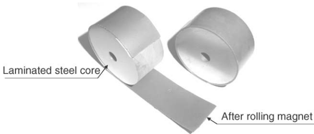
Fig. 5. External views of a radially anisotropic ring-shaped hybrid-magnets. The intended dimensions of the magnets are 50 mm in outer diameter and 1.05 mm in thickness.
